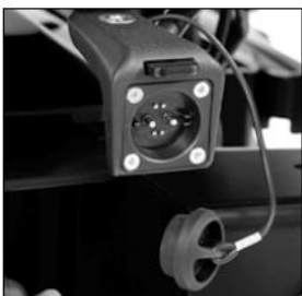
EU043 External magnetic charging receptacle
