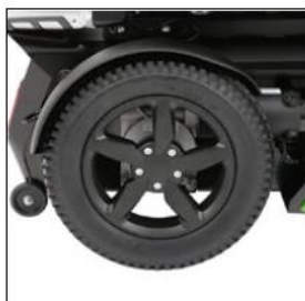
EA010 Splash guard for drive wheels
