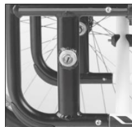
MA 114 Drive wheel adapter, permanently welded
