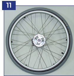
11 Rear wheel HOGGI light with drum brake
