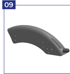
09 Aluminium fender with integr. brake system
