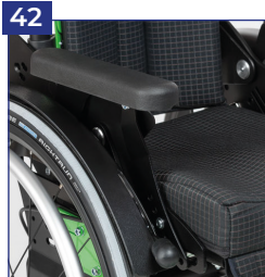
42 Armrests with tilt balancing
