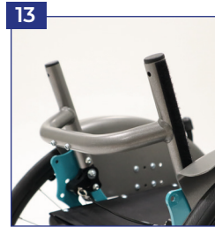
13 Back rest, retractable
