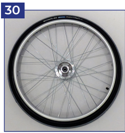
30 Pneumatic tires with drum brakes
