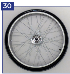
30 Pneumatic tires with drum brakes
