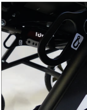
Attachment points, front according to ISO 7176-19
