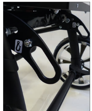
Attachment points, rear according to ISO 7176-19
