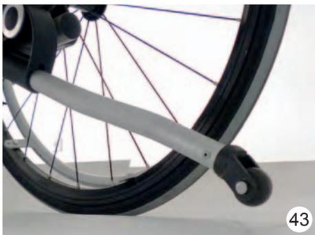
Picture 43 shows the position of the anti tip. The anti tip should be adjusted that it is 2-3 cm above the ground.
