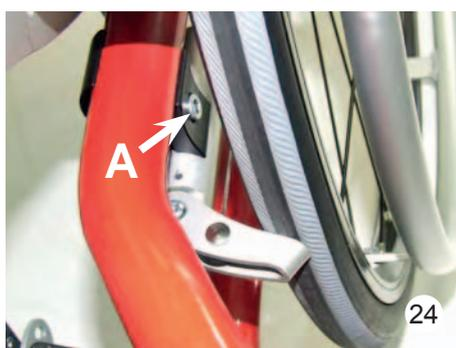
The brake shoe presses on the tires and grips it tightly. The brake shoe is, therefore, at a 90° angle to its holder (24). The brake shoe should overlap 3-5 mm to the middle of the wheel (24).
