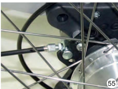
The brake force can be adjusted by the adjustment screw (55).
