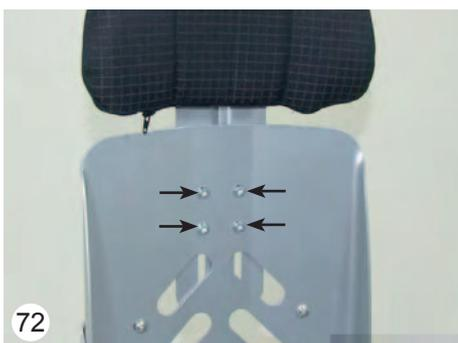
After loosening the four screws the headrest can be adjusted in the height (72).
