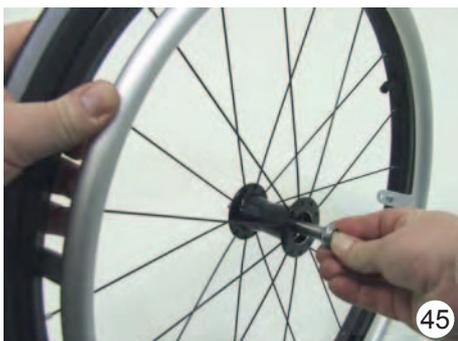
The rear wheels are removed by means of a quick-release mechanism. This reduces the volume of the wheelchair for transport:
