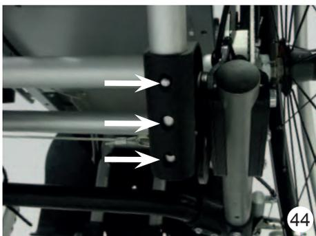
After pressing the snap button the length of the tubes can be adjusted in three positions (with respectively 2,5 cm distance).
