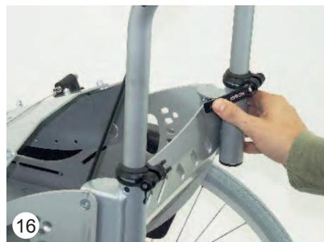
When the cam lever is open, its tension can be altered by adjusting the nut (17).
