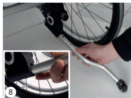
**SWINGBO-VTi** is equipped with two anti-tippers. The image (9) shows the „active“ position.
