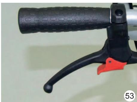
Each drum brake is operated by a brake lever (53).
