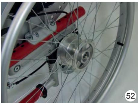
In addition to wheel lock and wheel lock (lever integrated in wheel guards), the SWINGBO-VTi wheelchair can be fitted with drum brakes.
