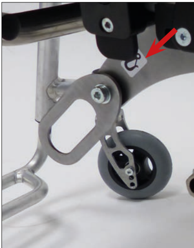
Attachment points, front according to ISO 7176-19
