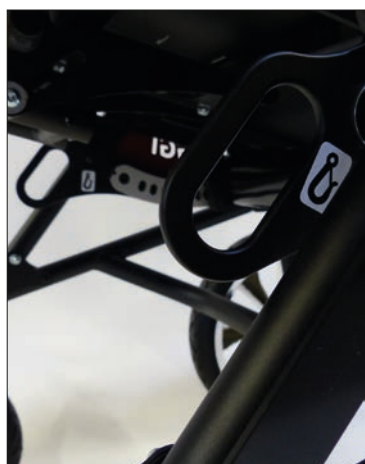
Attachment points, front according to ISO 7176-19
