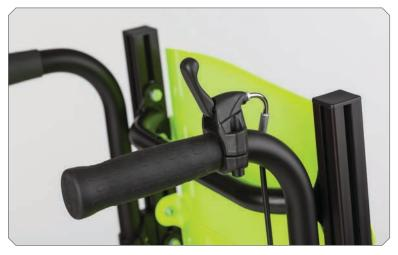
Release tilt in space mechanism.
